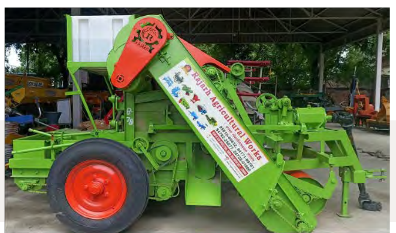
Nursery raising machine for mechanical transplanting
